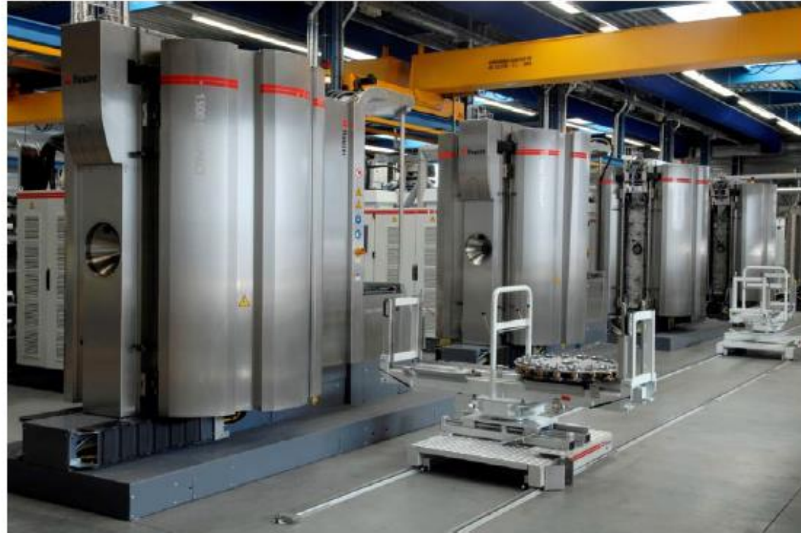
Industrial deposition system for the fabrication of DLC coatings for automotive parts and other applications. Each chamber contains six 1.6 m long electrodes. (Courtesy of Hauzer Techno Coatings)
