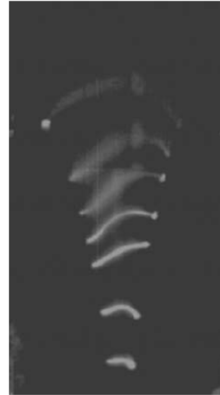
FIGURE 2.10 (a) Gliding arc electrode configuration with indication of the LTE and non-LTE region. (b) Superposition of snapshot images of a gliding arc discharge that illustrates the dynamic movement of the arc. (Reprinted with permission from Fridman, A., Plasma Chemistry , Cambridge University Press, Cambridge, 2008, © Cambridge University.)
